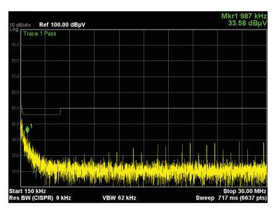
Figure 3. LT8610 Demo Circuit EMI Performance, Switching Frequency = 1MHz
