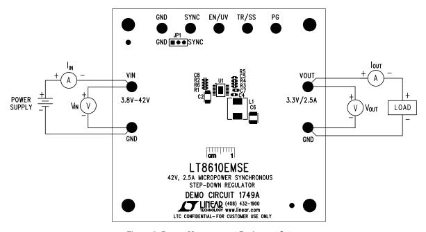
Figure 4. Proper Measurement Equipment Setup
