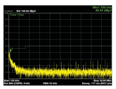
Figure 2. LT8610 Demo Circuit EMI Performance, Switching Frequency = 700kHz
