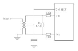
Figure 4. Transformer-Coupled Input
