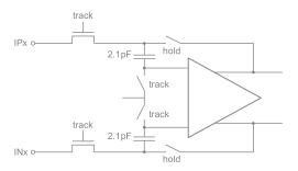
Figure 2. Input Configuration
