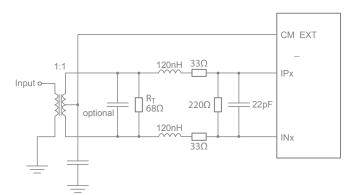
Figure 6. Alternative Input Network
