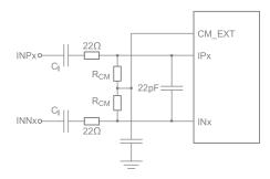
Figure 5. AC-Coupled Input
