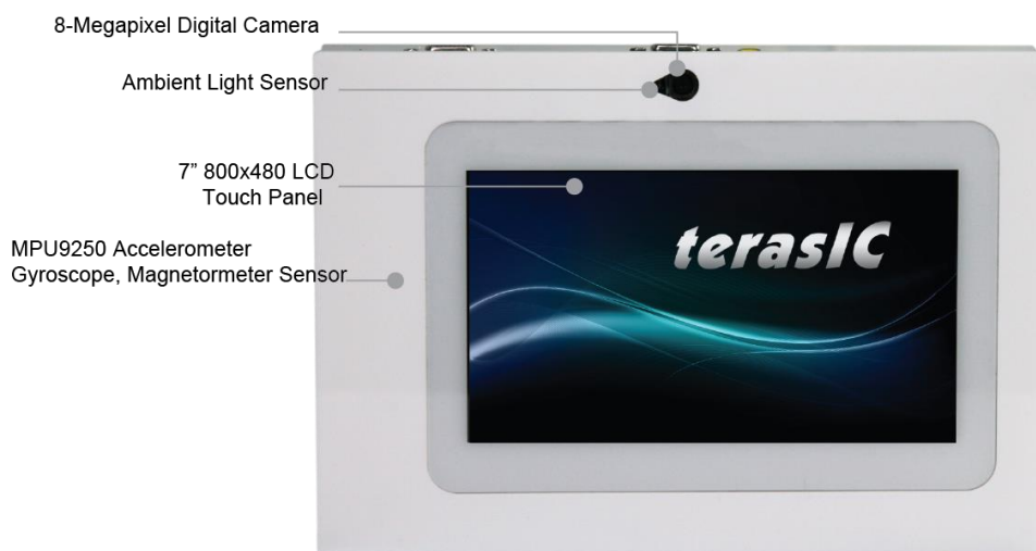
Figure 2-1 VEEK-MT2-C5SOC PCB and Component Diagram (top view)
