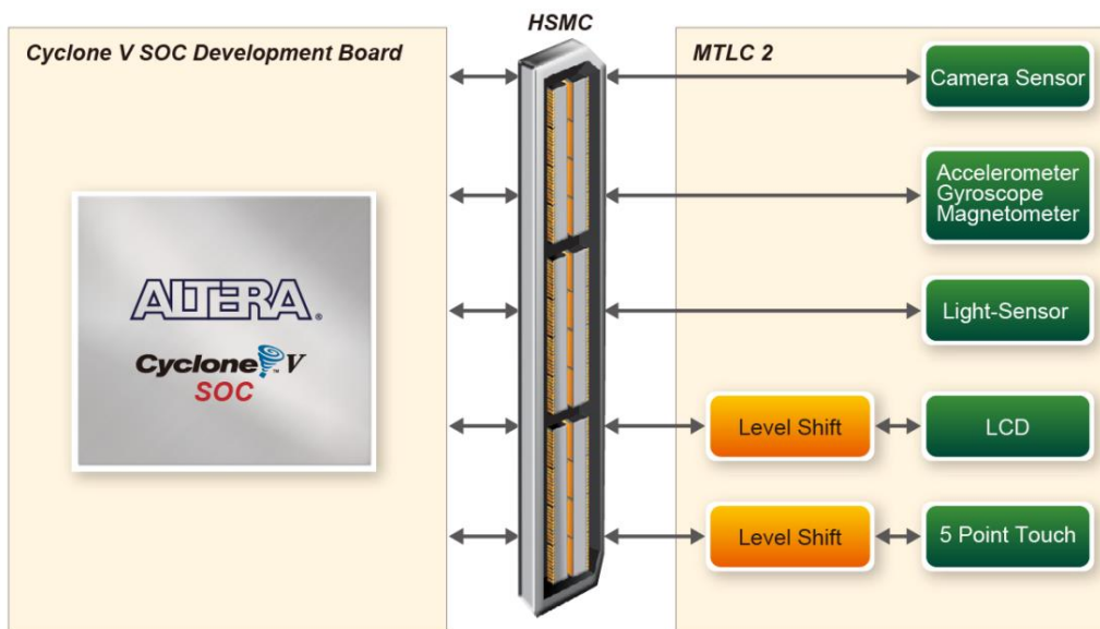
Figure 2-3 Block Diagram of VEEK-MT2-C5SOC
