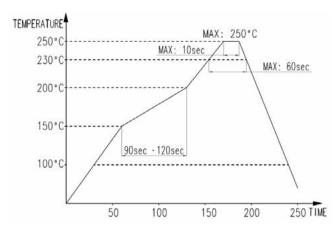
The temperature profile is based on the left conditions. In individual applications the actual temperature may vary, depending on solder paste type, volume/thickness and board size/thickness. Contact your solder paste and equipment manufacturer for specific recommendations.
