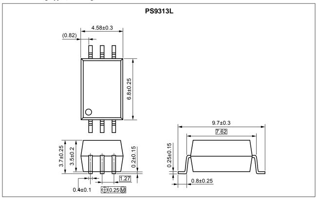
• Lead Bending Type For Long Creepage Distance (Gull-wing) For Surface Mount
