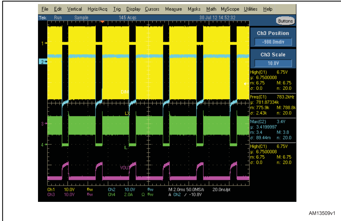
Figure 25: Inverting BB dimming operation
