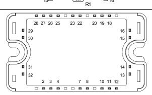
All multiple inputs and outputs must be shorted together Example: 13/14; 29/30; 22/23 ...
