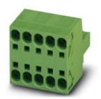
Plug component, Nominal current: 41 A, Rated voltage (III/2): 1000 V, Number of positions: 12, Pitch: 7.62 mm, Connection method: Spring-cage connection, Color: green, Contact surface: Tin
