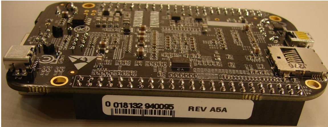
Figure 78. Third Phase Serial Number and Revision Location
