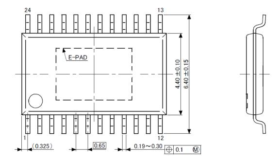
The heat sink is located on the back side and has dimensions of 2.85 mm  $\times$  4.05 mm.
