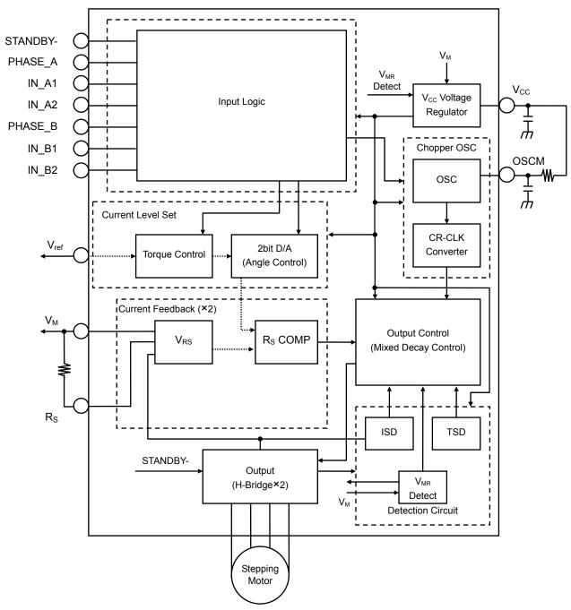
In the block diagram, part of the functional blocks or constants may be omitted or simplified for explanatory purposes.
