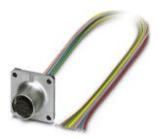
Sensor/actuator flush-type socket, 8-pos., M12, A-coded, front/square flange mounting, with 0.5 m TPE litz wire,  $8 \times 0.25 \text{ mm}^2$
